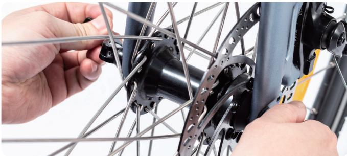
3. 2 Make sure the front wheel will not rub the brake pads when it is rotating under the condition of not pinching brake handle.
