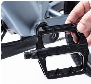
Tighten the right pedal clockwise and tighten the left pedal counterclockwise with the 15# wrench.
