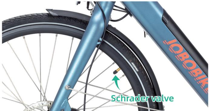
Check whether the tyres beads and tyres are evenly seated on the rims. Use a pump with a Schrader valve and pressure gauge to the recommended pressure indicated on the tyre sidewall.
