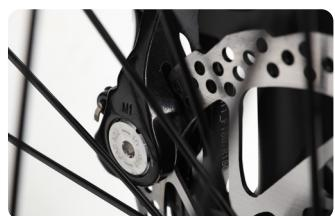
3.4 Screw the left and right nuts together with two wrenches and make sure the front wheel is fixed to the front fork tightly.
