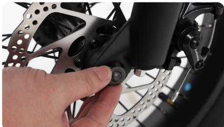
3.2 Put the wheel into the front fork groove.
