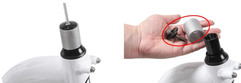
2.2 Install the handlebar stem on the front fork and tighten the bolt to the end.
