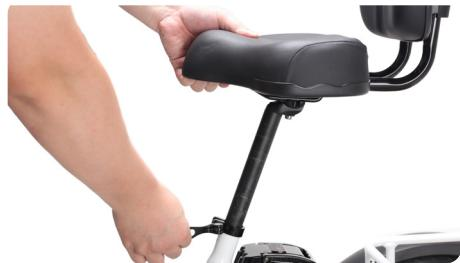
7.2 Close the buckle lever and make sure the lever is tightened enough when locking the saddle post.
